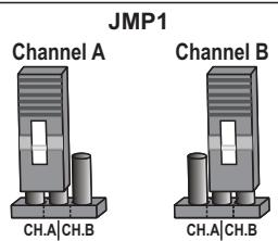
In this way, also if illuminating the receiver Rx2, the photocell Tx1 never realizes the alignment condition because Tx1 and Rx2 are configured on two different functioning channels.
