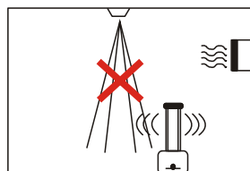
Do not install in the direction of sources of heat or air conditioners
