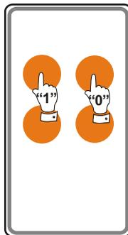
If the data entry is suspended for more than thirty seconds, the LED flashes for a few seconds and automatically exits the programming phase without changing the pre-existing code.
